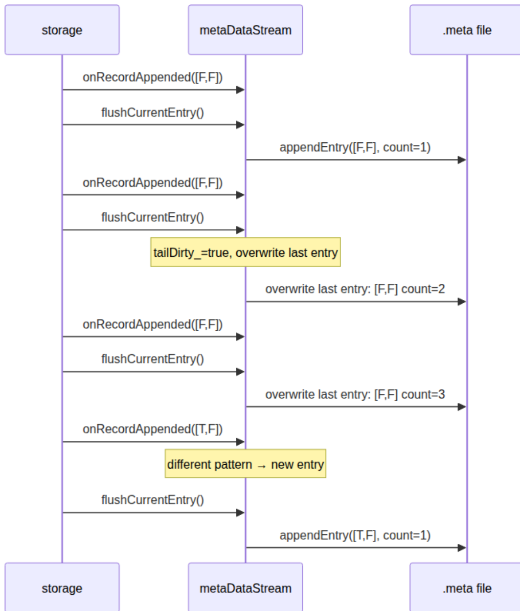
Fig. 17. The lazy-overwrite mechanism — overwriting the last .meta entry
